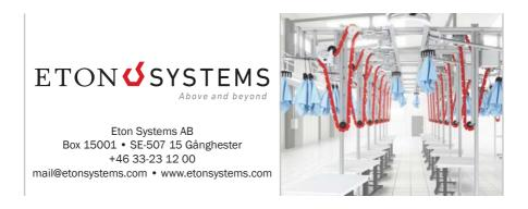
Eton Systems globally provides material handling systems consisting of individually addressable product carriers, automatically finding its way to the correct operation. The systems are designed to eliminate manual transportation and minimize handling, radically increasing the time for adding value to customer's products.
